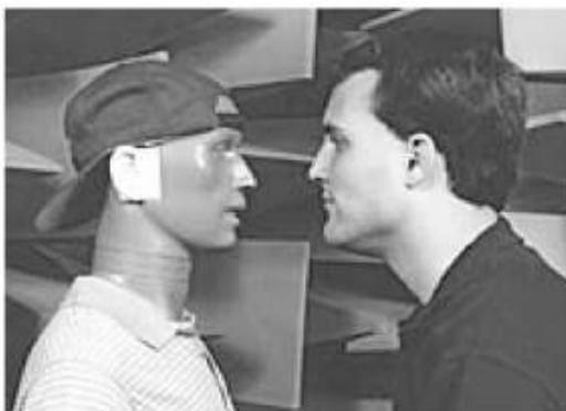
**Fig 7 :** KEMAR<sup>9</sup> dite Dummy Head
