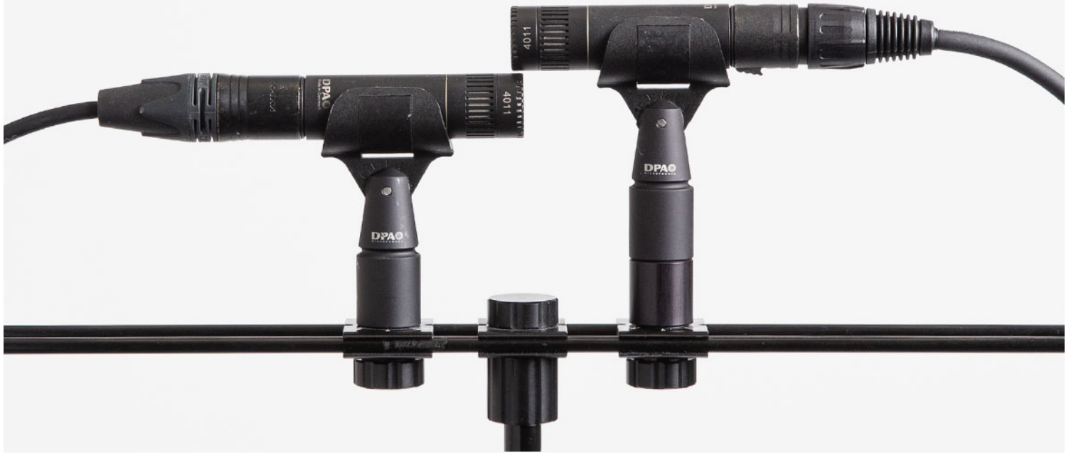
Fig. 13 Here, two cardioids replace a figure-of-eight microphone. Two microphone inputs are needed in principle. However, you can “cheat” by using a Y-sum cable with pin 2 and 3 reversed in one microphone connector.
