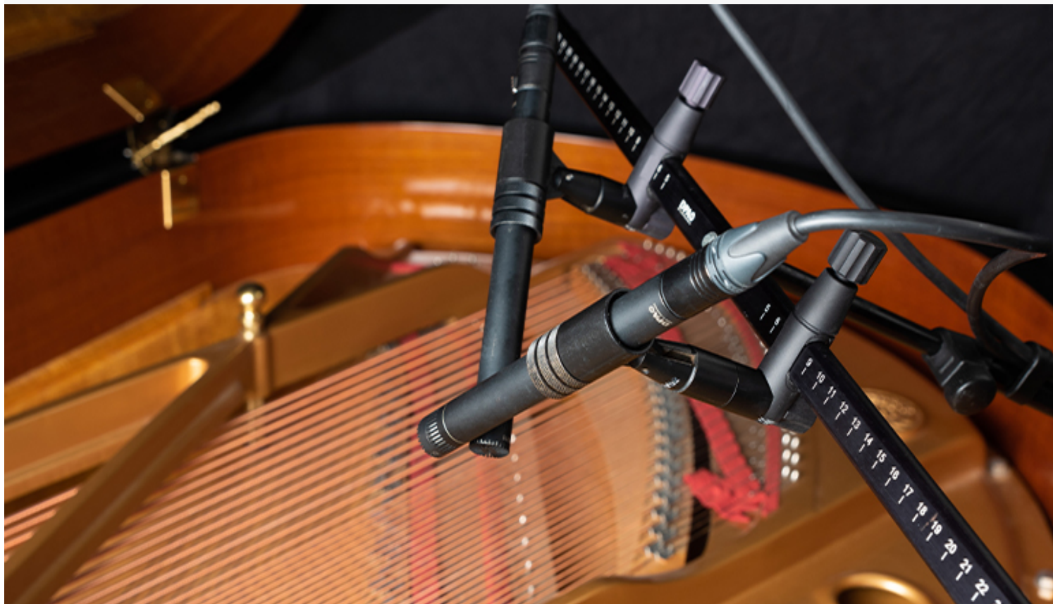
Fig. 9 Mounting the microphones closely but without any physical contact.
