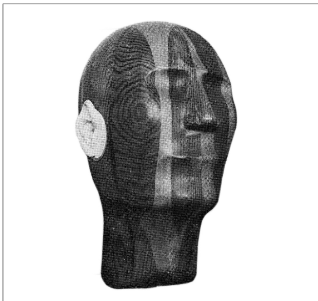
Figure 21. The wooden artificial head made by Kleiner [120].
