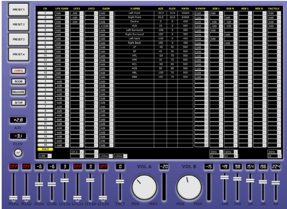
This screen shot shows input selection, audio routing, bass management, direct bass redirection and down mix for both listeners for the selected preset. A8 owners will be familiar with many of these functions, but just not seeing them on one screen. Unlike the A8, the input selection and speaker assignments now form part of the preset configuration.
