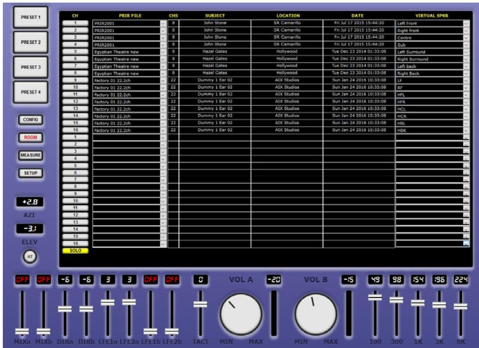
This screen shot shows the virtual room speaker set up menu for the selected preset. Each of the inputs can be assigned any virtual speaker from any PRIR file the user has stored in the A16, on the micro SD card, or, if connected to the internet, any PRIR or BRIR file the user has in their account in our Realiser Exchange website. This is a major improvement from the A8 which could only load entire PRIR files to presets.
