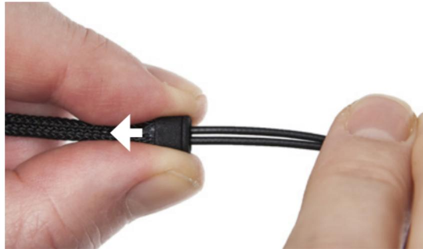
Before adjusting the frame size, you need to loosen the braided sleeving covering the cable. Remove the clothing clip, grab the bottom of the sleeving and pull it gently upwards, smoothing it up the entire length of the cable to make it loose at the top.
