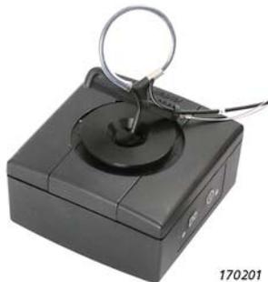
In-use level calibration of the binaural microphone set is performed using the supplied calibration adapter together with Sound Calibrator Type 4231. Using the adapter, the output level from the calibrator will be increased by 0.35 dB ±0.2 dB.
