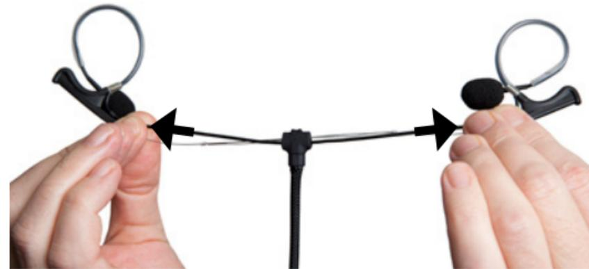
To increase the frame size, hold the cable and frame behind the earhooks and slowly pull the ear hooks away from each other to the desired size.
