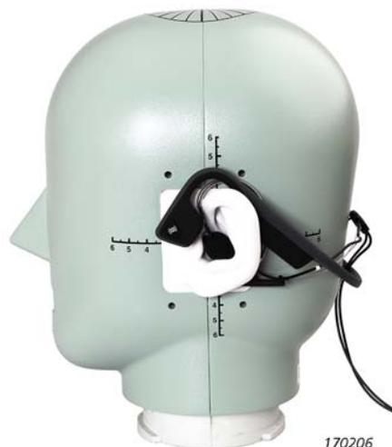
As the headphones are separate from the microphone headset, they can be effortlessly removed to perform measurements while the test subject is wearing a helmet and/or is exposed to high gravitational forces.
