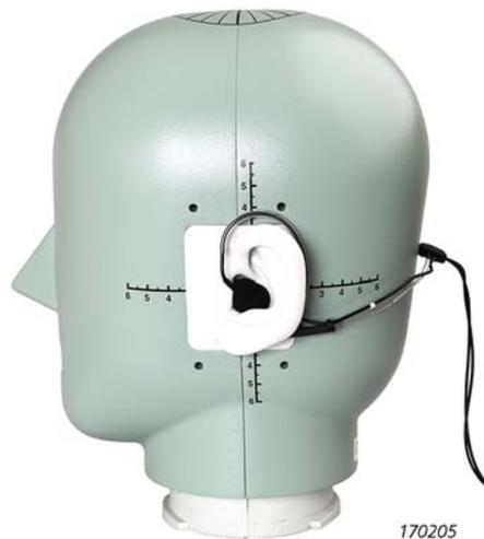
It comes with an ergonomic mount that wraps around the back of the user's head and ears. This mount can be easily adapted to suit any ear size and/or head shape for a secure yet comfortable fit. The individual microphone capsules sit in the concha of the ear, cushioned by the included foam windscreens (these are available in two different sizes to fit most users).
