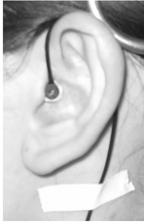
Figure 3. Blocked-ear-canal measurement with miniature microphone
