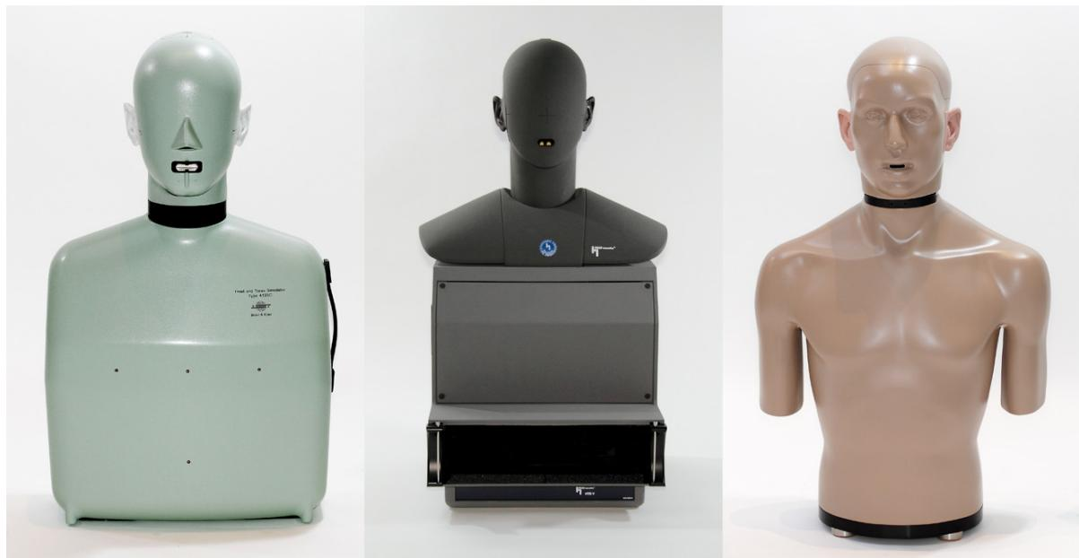
Figure 44: From left to right, Brüel & Kjær Type 4128-C, Head Acoustics HMS II.3 and G.R.A.S. KEMAR Type 45BM
