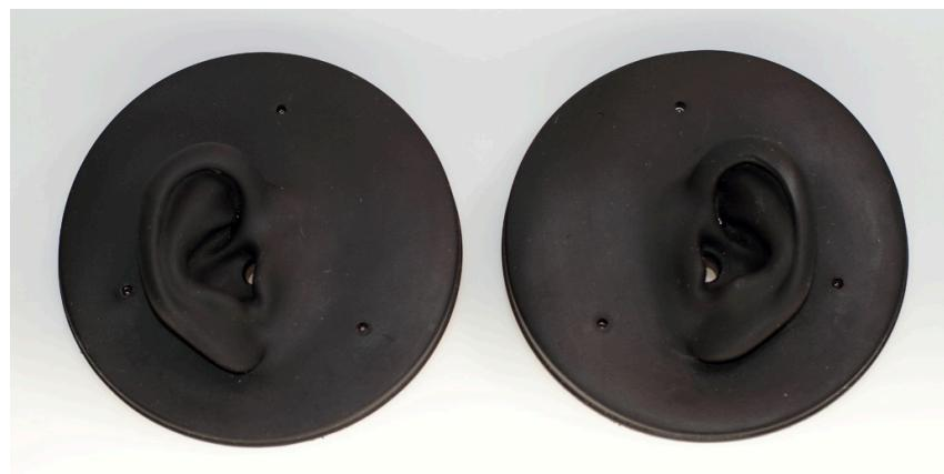
Figure 47: Right and left pinnae from Head Acoustics HMS II.3. Right/Left Pinna according to ITU-T P.57 Type 3.3, anatomically shaped.
