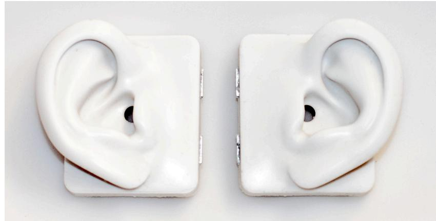
Figure 45: Right and left pinnae from Brüel & Kjær Type 4128-C HATS. Type numbers are DZ-9769 and DZ-9770 respectively.
