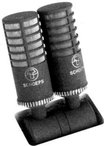
Feature: The angle between the microphones' axes can be adjusted without simultaneously affecting the stereo main axis. Due to the toothed wheels at the bottom end of the microphones, they always rotate equally in opposite direction to the main axis.
