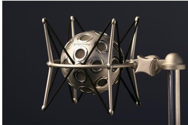
**Figure 3.1:** The em32 Eigenmike<sup>®</sup> spherical microphone array. *Photo used with permission from mh acoustics.*
